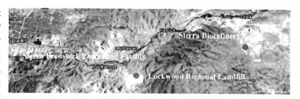
Sierra will convert approximately 175,000 tons per year of processed municipal solid waste ("MSW"), or household garbage, into approximately 11.0 million gallons per year of syncrude utilizing gasification and Fischer-Tropsch ("FT") technologies. The syncrude can then be processed into low-carbon transportation fuel products by standard refining subsystems. Sierra will be constructed in two phases,
