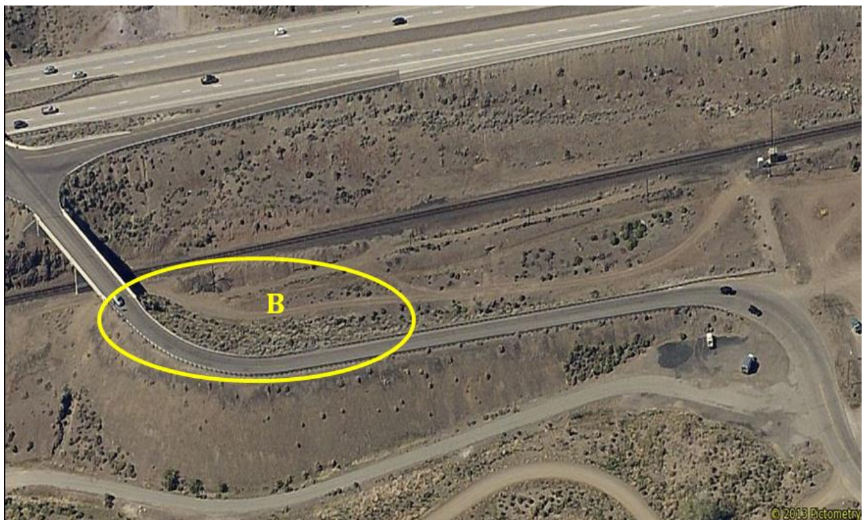
Figure 8.2-7: The images depict the existing infrastructure connecting Lockwood to Interstate 80. The image illustrates an on-ramp with substandard length for safe entry onto the interstate (A), and sharp and narrow curvature which inhibits safe two-way vehicle and truck travel (B). (Source: Storey County Planning Department, 2015)
