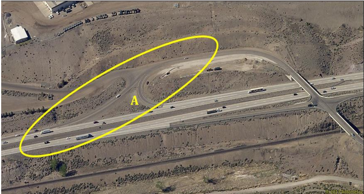
Figure 8.2-7: The images depict the existing infrastructure connecting Lockwood to Interstate 80. The image illustrates an on-ramp with substandard length for safe entry onto the interstate (A), and sharp and narrow curvature which inhibits safe two-way vehicle and truck travel (B). (Source: Storey County Planning Department, 2015)
