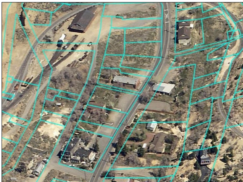
Figure 8.2-3: Virginia City aerial with lot lines. This image, also included in Chapter 3 Land Use, illustrates existing traveled ways located significantly outside of right-of-ways, and right-of-ways which conform very little to area topography, railroads, and other ground conditions. (Source: Storey County Assessor's Office, 2015.)
