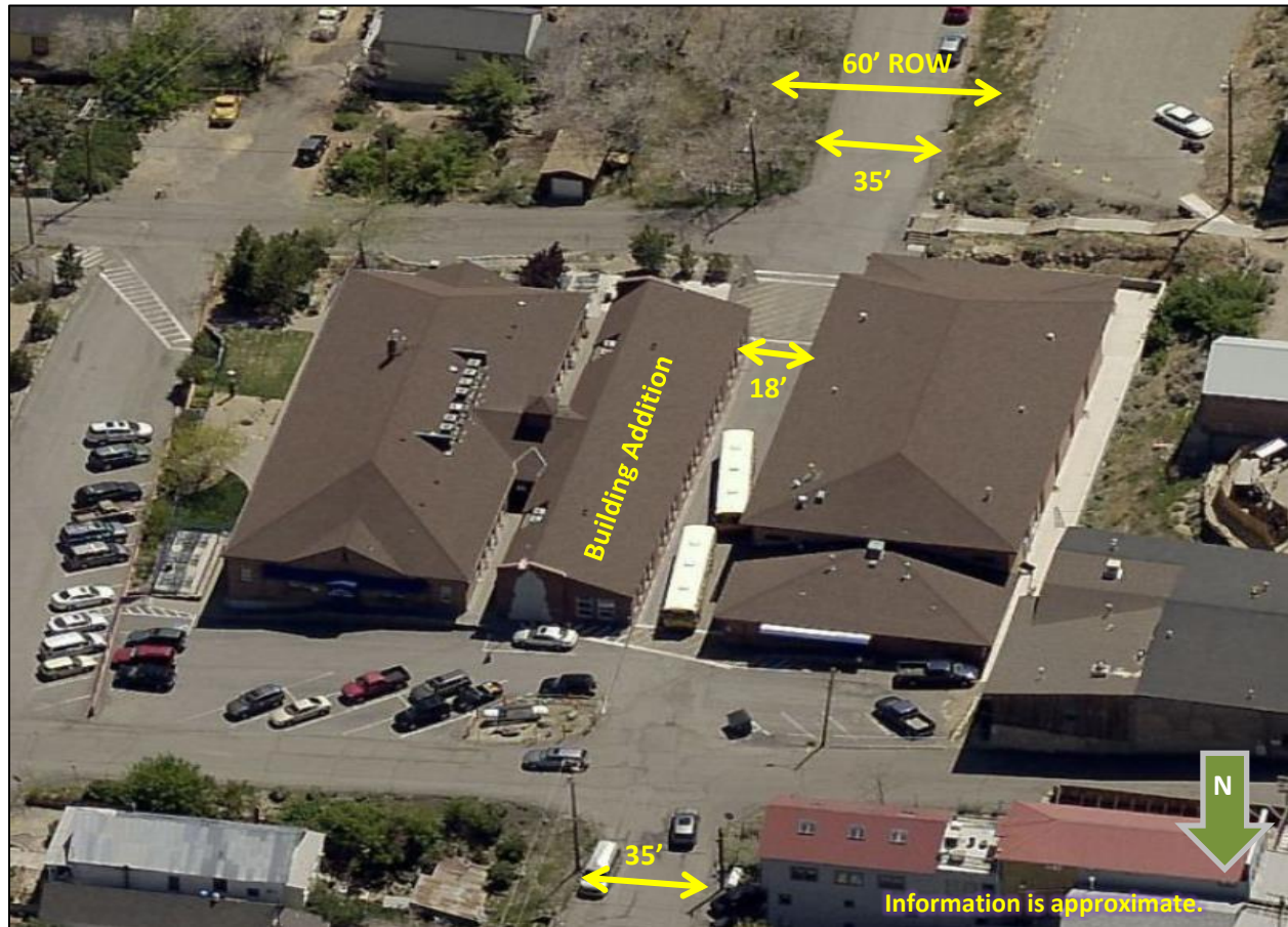
Figure 8.2-5: Bottleneck by middle school. The image illustrates the bottleneck that was created when the addition to the Virginia City Middle School was built in the “D” Street right-of-way. The remaining street width is not sufficient to facilitate regular heavy traffic loads (Source: (top) Storey County Planning Department, 2016; (bottom) Storey County School District, 2016).
